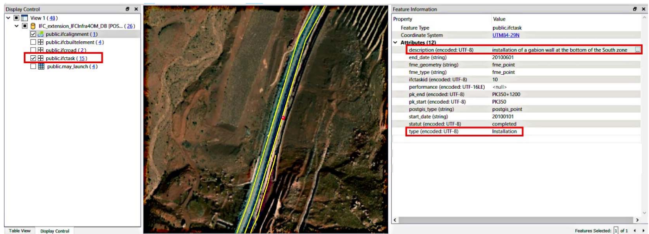
Figure 10. O&M information extraction from IFCTask class and its geolocation on the IFCAlignment entity.
